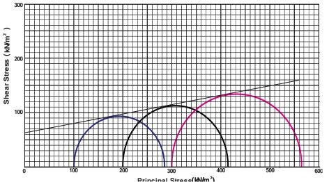
Principal Streed (MV/m<sup>2</sup>) FIGURE 4. TYPICAL PLOT OF MOHR CIRCLES AND ENVELOPE OF UPPER CLAYS
