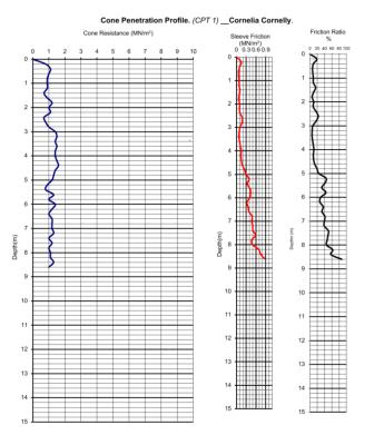
FIGURE 5. CONE PENETRATION PROFILE OF BOREHOLE 1
