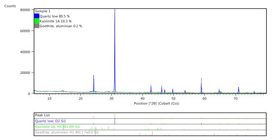
FIGURE8.Sample diffraction trace of clay minerals
